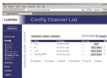
The L-IP Router connects twisted pair channels (TP/FT-10 or TP/XF-1250) with the Ethernet/IP channel (IP-852) in LonMark Systems. L-IP routes CEA-709 packets through an IP based network such as a LAN (Ethernet), an Intranet, or even the Internet. The L-IP connects to the IP network via a 100Base-T Ethernet port.
