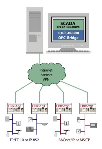
The diagram shows a SCADA (Supervisory Control and Data Acquisition) system. It is installed on a PC and connected to LonMark systems and BACnet networks via the L-INX Automation Servers. The SCADA system uses the protocol OPC DA (COM/DCOM) to monitor and control process data. The L-INX Automation Servers are using the OPC XML-DA communication protocol.
